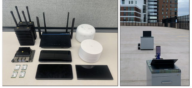
Fig. 2. Overview of initiating and responding stations (left), and our Wi-Fi FTM accuracy evaluation setup (right) of Appendix A.
