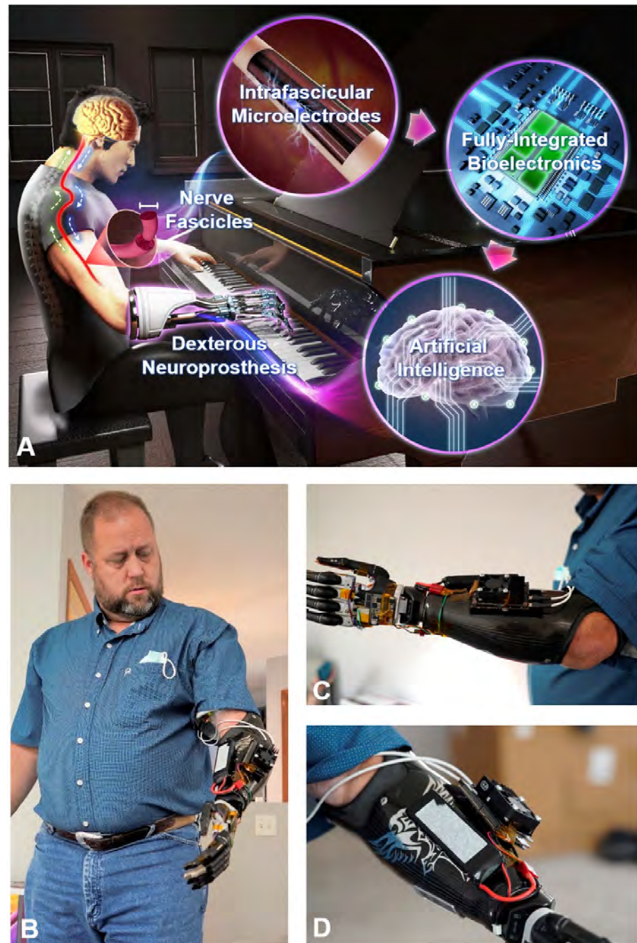
Figure 1. (A) Artistic concept of the next-generation dexterous and intuitive neuroprostheses. Reproduced from [23]. © IOP Publishing Ltd All rights reserved. (B)–(D) Here we present the implementation of a functional, fully portable, self-contained prototype toward this goal.
