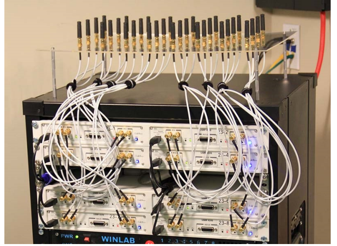
Fig. 3: Massive MIMO mini-racks. 4 such racks on each corner of the ORBIT Testbed. Each rack consists of 8 USRP X310s and 32 antennas
