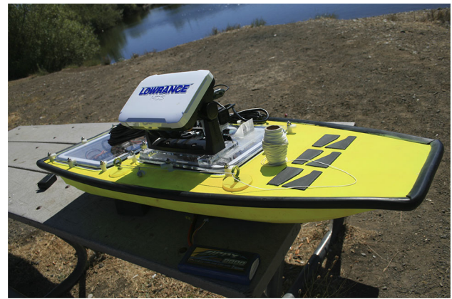
Fig. 12 Platypus Lutra autonomous boat with lowrance depth sonar used in field trial experiments (Platypus, LLC 2014) (Color figure online)
