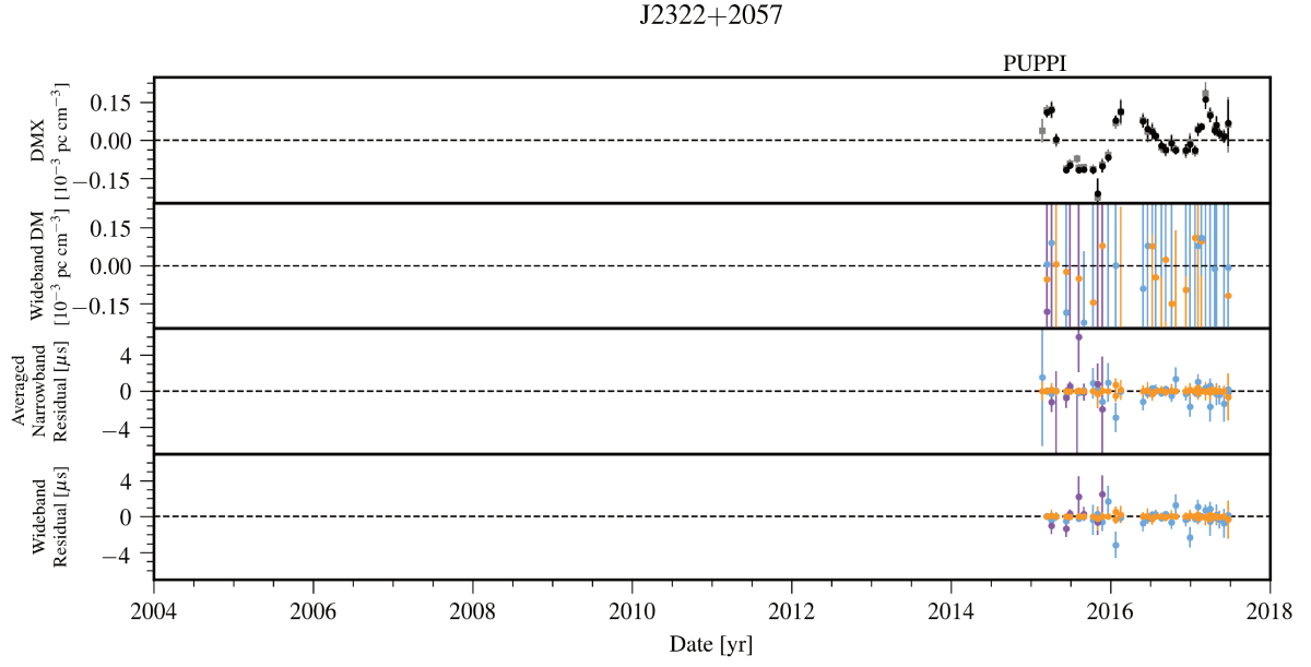
Figure 55. Timing residuals and DM variations for J2322+2057. See Appendix C for details. DMX model parameters from the wideband (black circles) and narrowband (grey squares) data sets are shown in the top panel. Colors in the lower panels indicate the receiver for the observation: 430 MHz (Orange), 1.4 GHz (Light blue), and 2.1 GHz (Purple).
