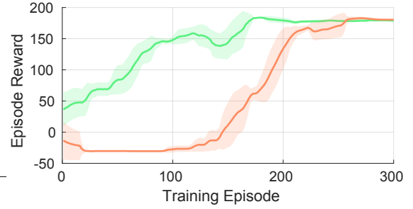
Fig. 8. Running average of reward and its standard deviation for the cartpole swingup task. The RTS+RL framework (green) is able to more rapidly converge to a high reward policy when compared to a baseline RL approach (red).
