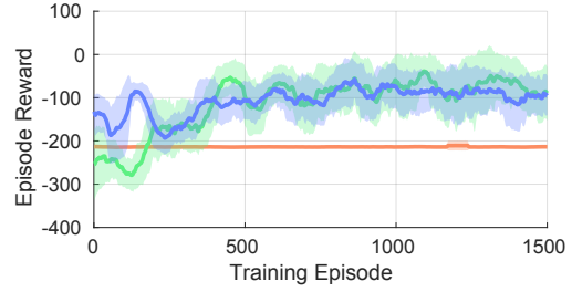
Fig. 5. Running average of reward and its standard deviation during training for the drone obstacle tunnel. Our RTS+RL framework (green) learns to navigate the random obstacle tunnels, whereas the discrete version (blue) does not achieve as much reward. The baseline RL approach (orange) struggles to accumulate reward, and instead learns to collide with obstacles
