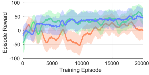
Fig. 3. Running average of reward and its standard deviation during training for the car lane change task. The proposed RTS+RL method (green) achieves high reward compared to a discrete version of the same method (blue) and a baseline RL approach (orange). Baseline RL had collisions in 40.2% of episodes, whereas RTS had none.
