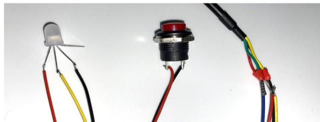
Fig. 31. Wiring on the LED (left), button (center), and SHT-30 Sensor (right).
