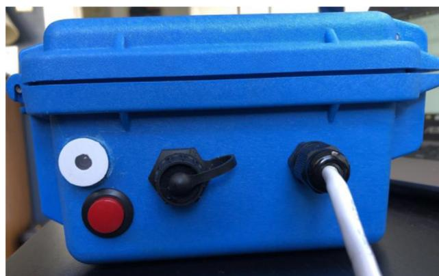
**Fig. 22.** The completed left side of the Pelican Case with LED plug, button, micro-USB port, and PG7 cable gland (the CAT5 cable in the cable grip of hole D will be implemented later).
