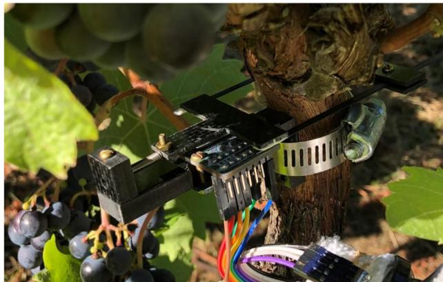
**Fig. 57.** Dendrometer prototype installed on grapevine at OSU Woodhall III Vineyards. Note there are small differences in the wiring setup and fasteners from those described here.
