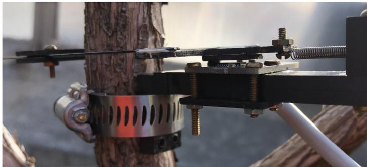
**Fig. 53.** A hose clamp holds the dendrometer on a stem or vine by wrapping around the Vine Contact Mount and tightening against the vine.
