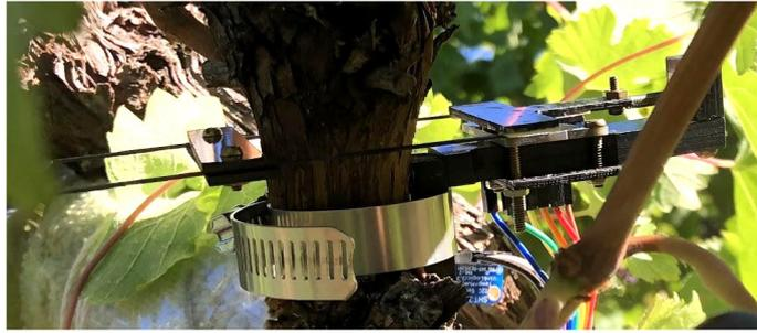
**Fig. 55.** Dendrometer successfully installed on a grapevine (note the wiring is different from build guide).
