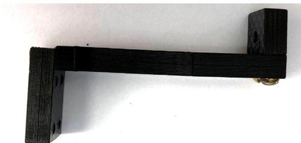
**Fig. 14.** Spring Hold (right) attached to the Long Body (center). The Vine Mount (left) is attached from the previous step.
