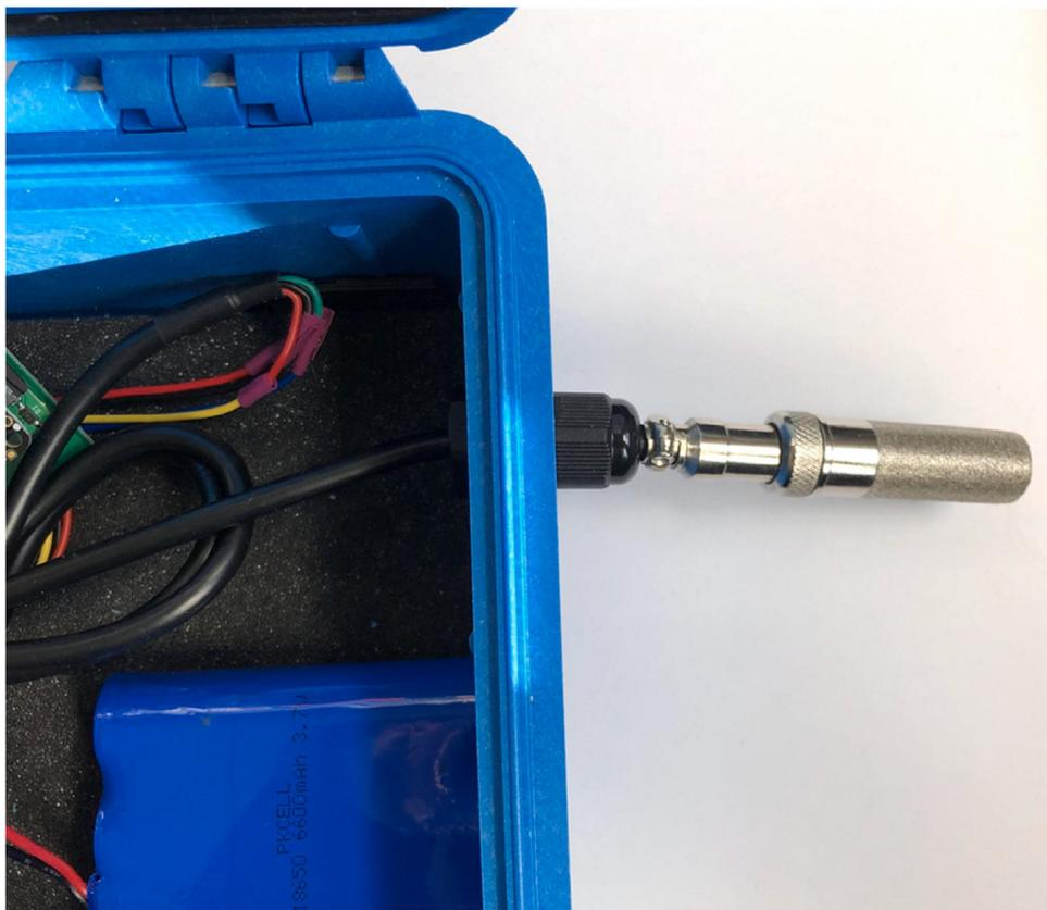
Fig. 20. The SHT30 with the sensor end on the outside (protruding from the black cable grip) and the cable on the inside of the Pelican Case.
