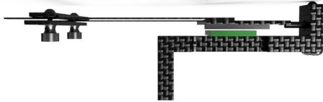
**Fig. 52.** Dendrometer orientation without the vine. Stem or vine will be in between the Sandwich Grip and Vine Magnet Mount when installed.
