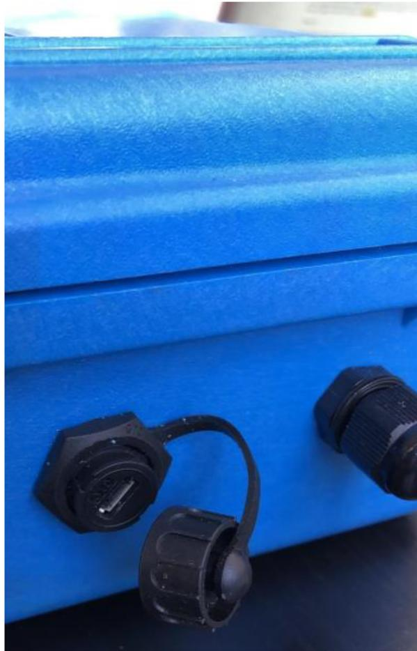
**Fig. 21.** The USB port (with the cap off) on the left side of the Pelican Case.
