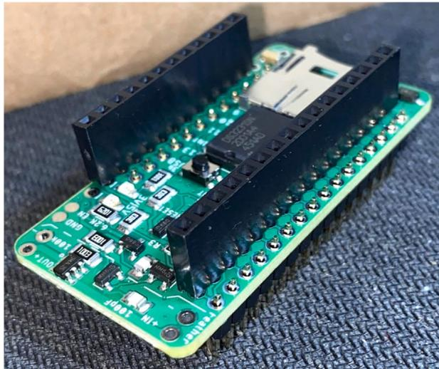
Fig. 23. Hypnos with a set of stacking headers and male headers.
