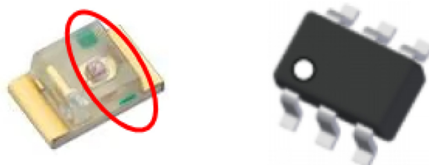
Fig. 5. Polarity Indications (Green lining on LED and circle in corner for large P-Channel MOSFET). (For interpretation of the references to colour in this figure legend, the reader is referred to the web version of this article.)
