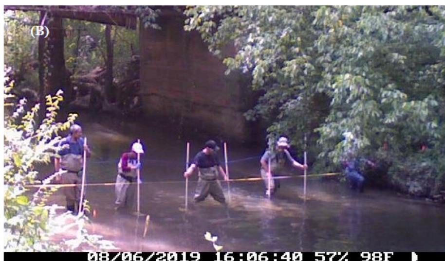
Fig. 2. Illustrative design of the thermal sensor array on the poles connected by 1-m long rope (A), and photograph of the temperature sensor array (B) during operation of the in-stream temperature survey conducted by a 6 person team moving the poles from downstream to upstream while measuring temperatures every 1-m along the stream reach length.
