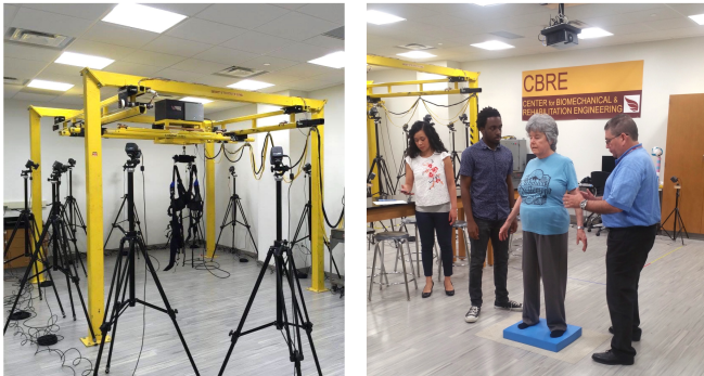
Figure 1. NaviGaitTor harness system (left); Administering BESS assessment (right)
