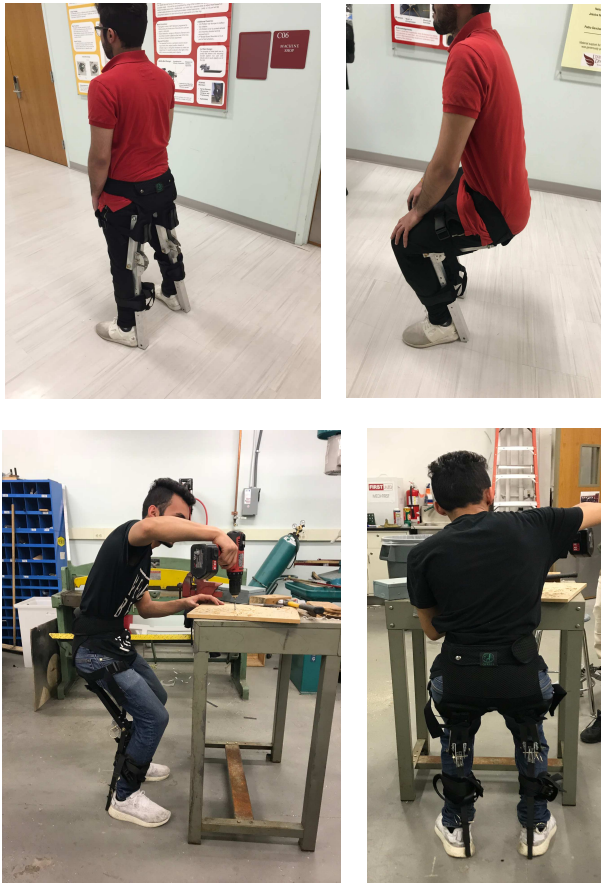
Figure 3. Chairless Chair Exoskeleton: Top - Initial Design Prototype #1 made out of aluminum; Bottom - Final Design Prototype #2 made out of carbon fiber.
