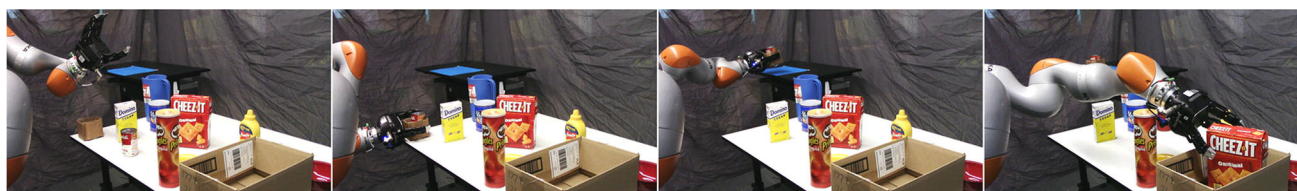
Fig. 1 Multi-stage delivery task: place the soup in an open-top box and deliver it, then deliver the Cheez-Its to a second delivery location. To avoid spills, a pose constraint is enforced while the soup is being delivered in the open-top box
