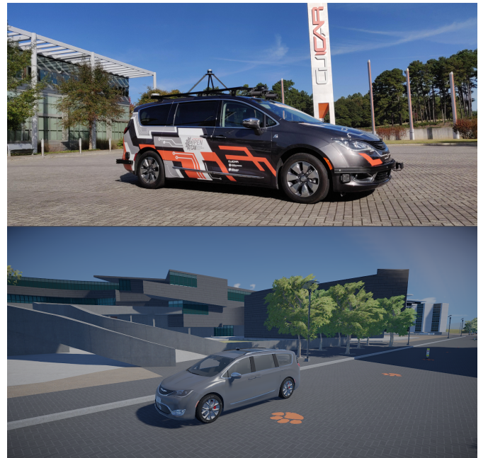
Figure 3: The OpenCAV vehicle in comparison to its digital twin
