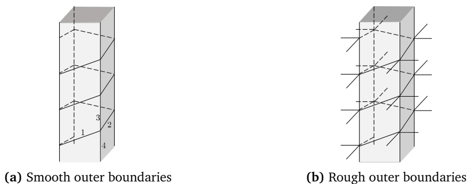
Figure 17: The minimal structure of a smooth screw dislocation.
