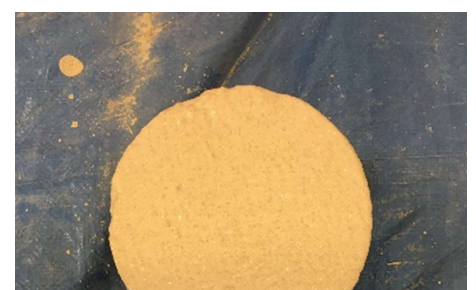
Figure 13. The coating sent by Decorative Paving Solutions, with parts A and B, and the colorant.
