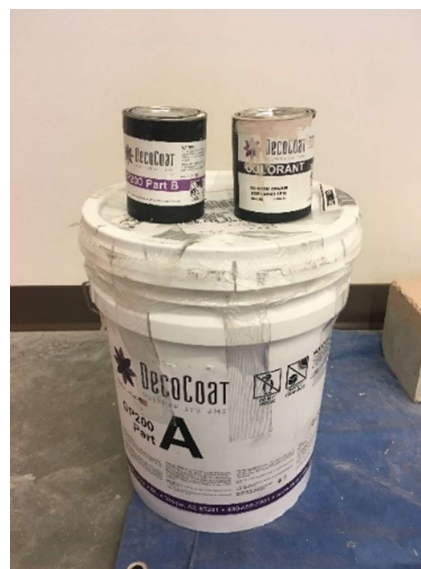
Figure 13. The coating sent by Decorative Paving Solutions, with parts A and B, and the colorant.
