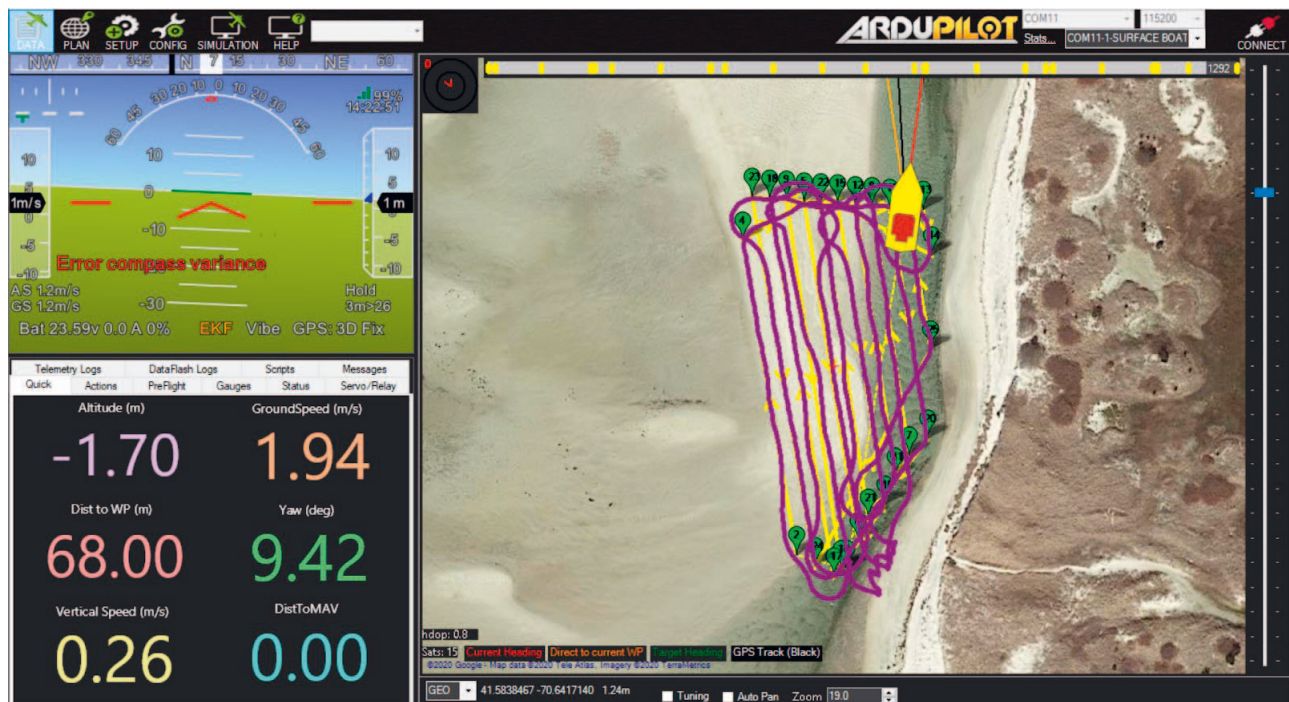
Figure 4. User interface of Mavlink, the program used to control the Ardupilot autonomy and track generation. This screen shows the display of the ground control station when the vessel is running a survey mission; in this case, a survey completed in Great Sippewissett estuary. This image provides a sense of what it is like to work with the vessel during a survey, including the map of the desired track, the actual vessel position, and relevant numbers such as distance to waypoint and vessel speed.
