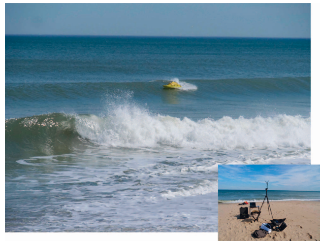
Figure 13. (Main figure) The vehicle underway conducting a turn at the near-shore end of a survey line in moderate breaking waves. (Inset figure) the highly portable control station set up on the beach within visual range of the vessel.
