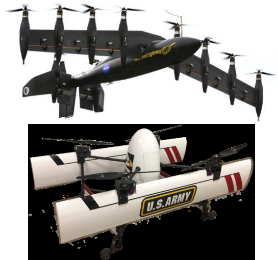
Figure 1: Novel eVTOL aircraft using multirotor configurations: (top) NASA GL-10 tilt-wing and (bottom) Army CRC-20 biplane tailsitter. Credits: NASA Langley/David C. Bowman and Ref. 1.
