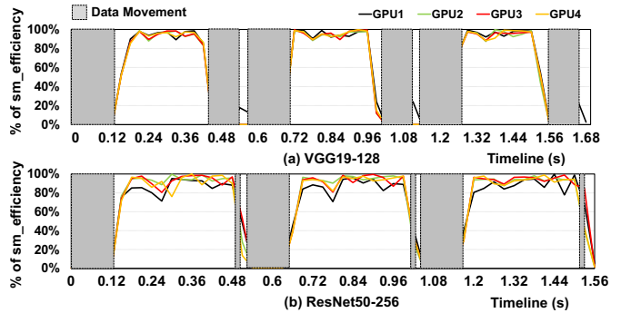
Fig. 5. Timeline results of GPU utilization for three batches during baseline training on Server A. (a) Results for \langle \text{VGG19}, 128, 4 \rangle . (b) Results for \langle \text{ResNet50}, 256, 4 \rangle .
