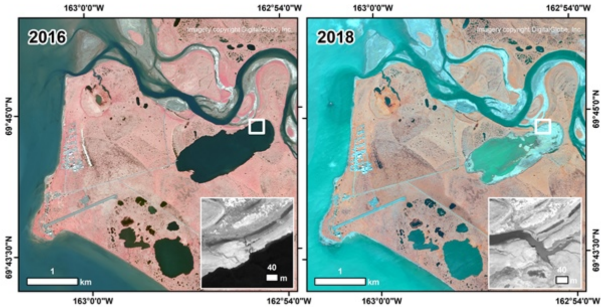
Fig. 2. The drinking water source lake in Point Lay, Alaska, catastrophically drained in fall 2016 because of permafrost degradation. The drainage was a result of bank overtopping and thermal erosion of an ice wedge (surface flow as opposed to subterranean drainage). The small inset shows the thermo-erosional gully that developed during the lateral drainage event. Drainage of thermokarst lakes in the Arctic is a natural process that is increasing in frequency because of climate change (Nitze et al. 2020), which is enhancing hazards in lowland permafrost regions (Arp et al. 2020).
