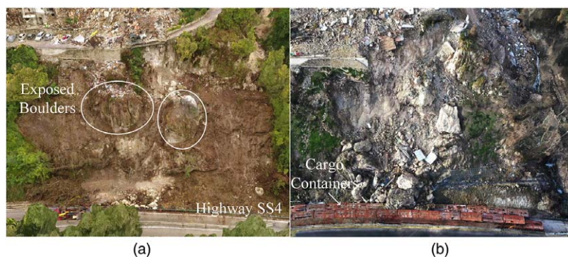
Figure 8. 3-D mesh model images of the largest observed debris slide below the village of Pescara del Tronto following the (a) 24 August and (b) 30 October events.
