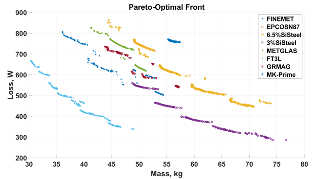
Fig. 8. Pareto-optimal front mass vs loss
