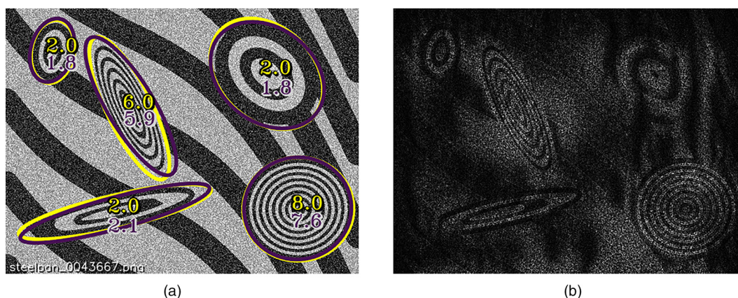
FIG. 4. (Color online) Sample fake images, showing ground-truth bounding ellipses and ring counts (upper values, light yellow) and those predicted by the network (lower values, dark purple). Top: original style of fake image, from FakeLarge dataset. Bottom: same fake image with “real” style transferred via CycleGAN (Ref. 42), from CGLarge dataset.
