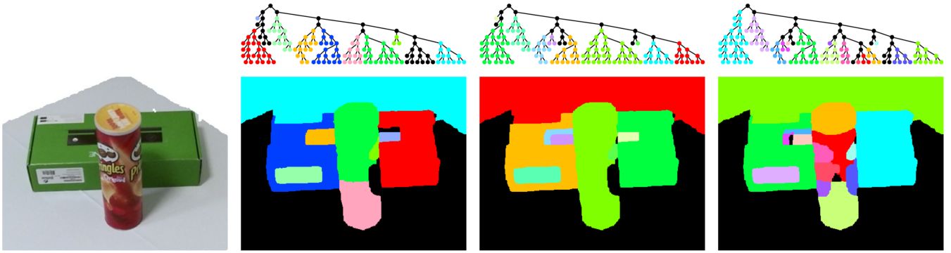
Fig. 3: Sampled tree cuts and their resulting image segmentations. The segmentation trees have been truncated for clarity; the full size is approximately 1000 nodes.
