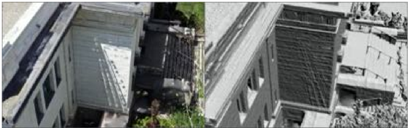
Figure 4. (Left) Shadow drift visible on the Maeser building May model (not used in final model). (Right) Geometric error in the mesh visible via a shaded geometry view of the model.
