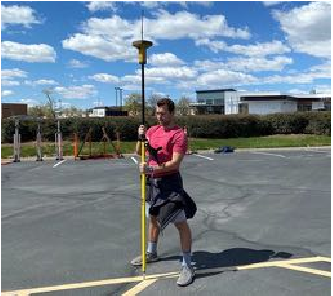
Figure 8. Topcon GR-3 GPS configuration used for gathering GCPs.
