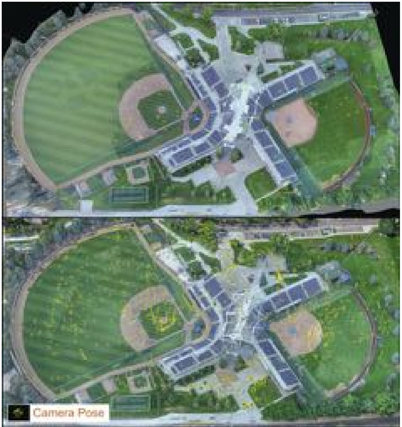
Figure 19. The baseball field rendered with all automated and manual photos (1458) [bottom] and the field rendered only using the 152 optimized photos [top].
