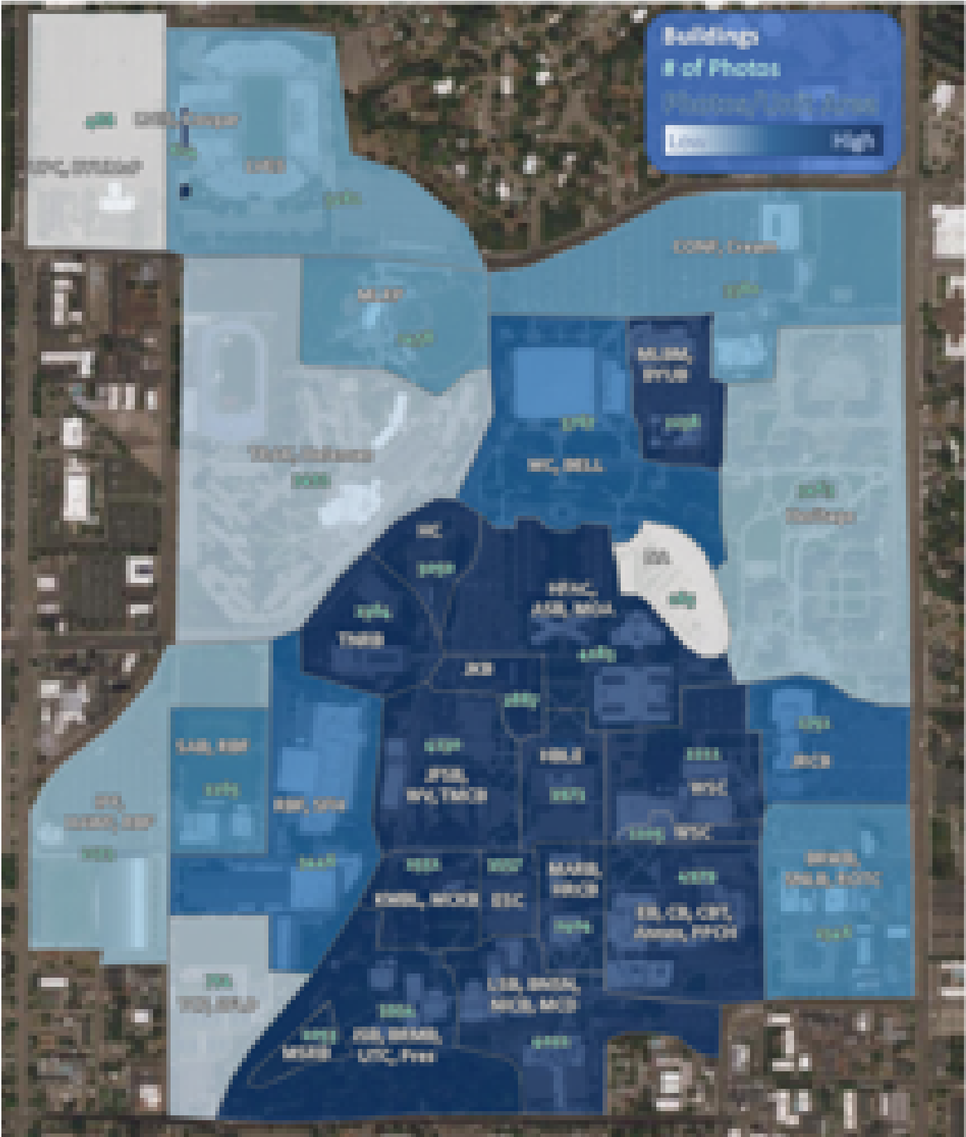
Figure 6. Areas depicting the original individually aligned models used to create the whole campus model after merging. Numbers refer to the quantity of photos used in each area. Colors correlate with the number of photos per projected area in the model with white relating to a low number of photos per unit area and blue a high number of photos per unit area.
