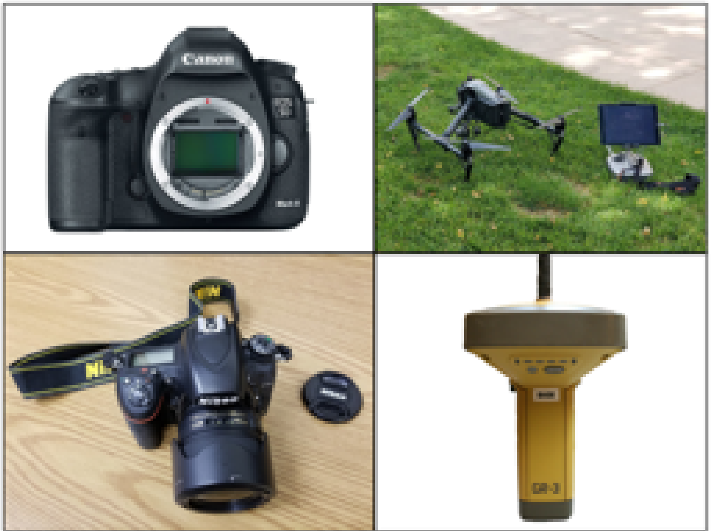
Figure 3. Equipment used for data collection. ( Top Left ) Canon EOS 5D Mark III, ( Bottom Left ) Nikon D750 with 35mm lens, ( Top Right ) Inspire 2 equipped with a Zenmuse X4S camera, and ( Bottom Right ) A GR3 Topcon GPS receiver.
