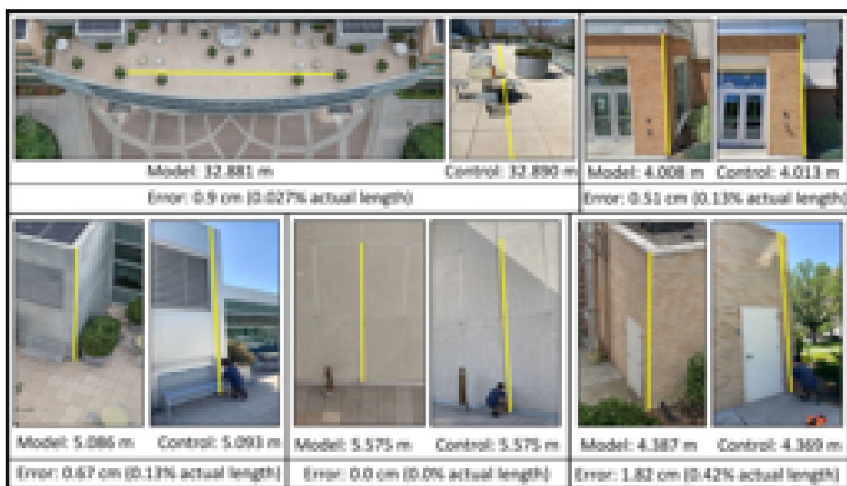
Figure 16. Five of the twelve relative model accuracy measurements displayed with a model screenshot on the left and a photo of the actual area on the right. Average model accuracy was 0.65 cm or 0.145% of the actual measuring distance.
