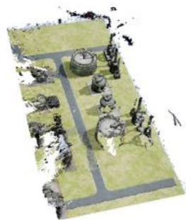
Figure 25. Iteration 2 failed to capture additional features, increasing the average GSD.
