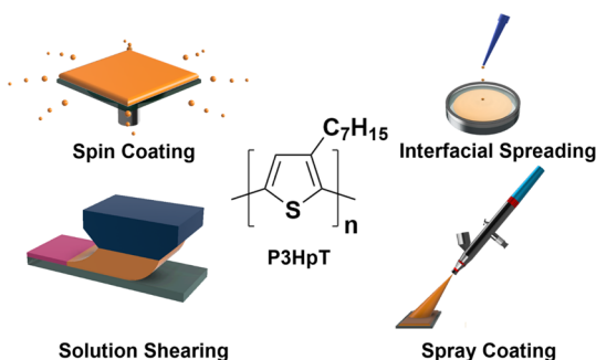
Figure 1. Films of P3HpT were cast using four different deposition processes: spin coating, interfacial spreading, solution shearing, and spray coating.
