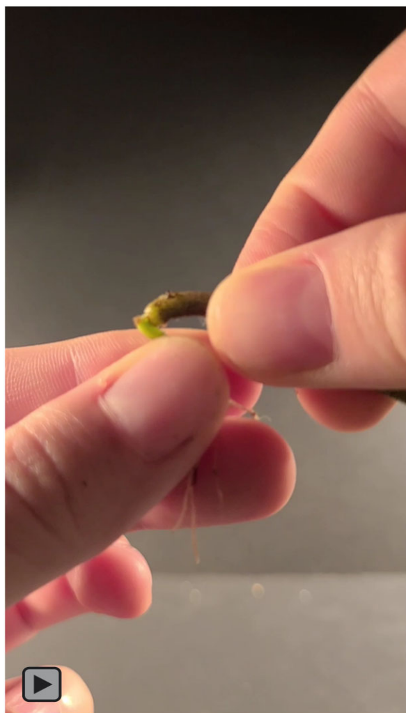
Movie 3 Bend test of heterografted tomato:pepper 30 DAG (supports Figure 1 ). Representative hetero-grafted tomato:pepper is bent from the rootstock and scion to test graft junction integrity. Around 92% of these plant could be broken at the graft junction. N = 12 .
