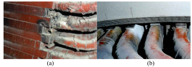
FIGURE 4. (a) Corona discharge at the slot outlet causes single phase ground fault on a 10kV three-phase asynchronous motor [18]; (b) Marks of corona discharge at the slot exit of a 2000kW/6kV high voltage motor [5].
