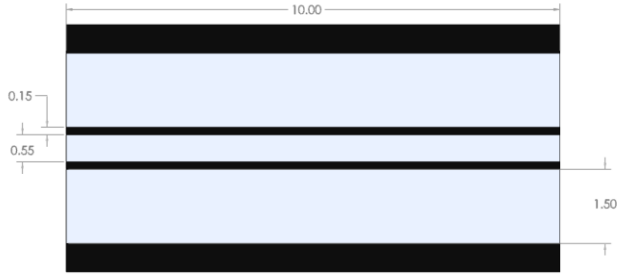
Fig. 2. CPW designed dimensions, in mm.
