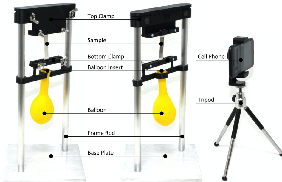
FIGURE 2. Hands-on mechanical test device. Rear view (left) and front view (right) with part labels and cell phone with tripod.
