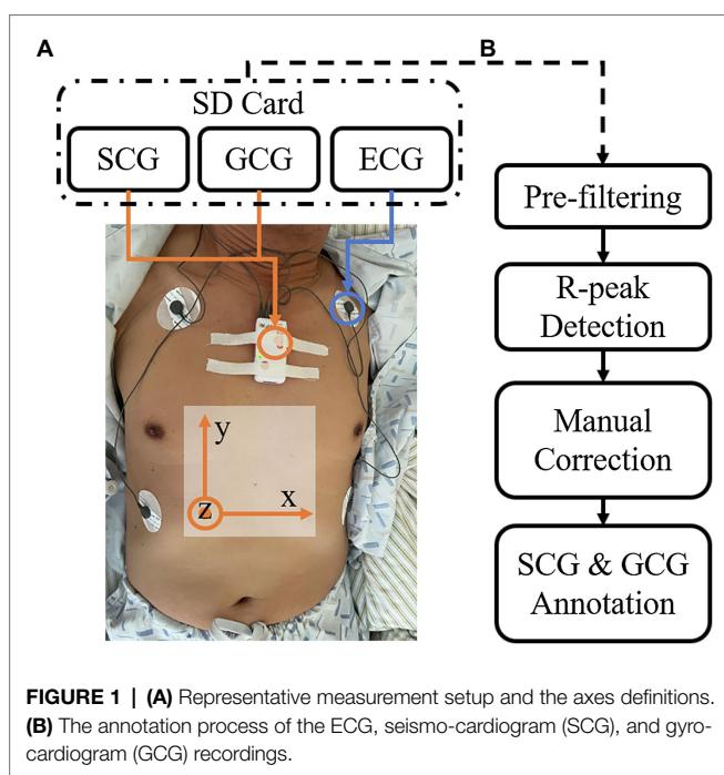
**FIGURE 1 | (A)** Representative measurement setup and the axes definitions. **(B)** The annotation process of the ECG, seismo-cardiogram (SCG), and gyro-cardiogram (GCG) recordings.
