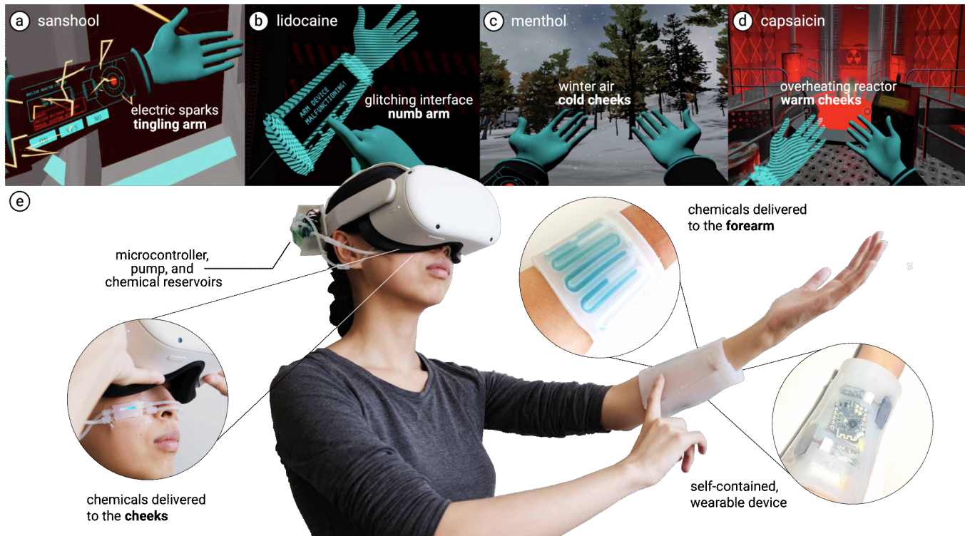
Figure 1: We propose a novel haptics approach, which we call Chemical Haptics , based on delivering topical stimulants to the user’s skin. Upon absorbing these stimulants, receptors in the user’s skin are chemically triggered, rendering distinct haptic sensations. To explore our approach in interactive contexts, such as VR, we engineered a self-contained wearable that delivers liquid stimulants. Here, it allows this VR user to feel four haptic sensations: (a) Sanshool creates tingling, which renders electric sparks emitted from a “short-circuiting” touchscreen on the arm; (b) Lidocaine creates numbing, which renders a malfunctioning arm interface by reducing tactile feedback as the user taps the buttons; (b) Menthol creates cooling, which renders cold winter air on the face; finally, (d) Capsaicin creates warming, which renders the hot air on the face from a nuclear reactor on the brink of meltdown.
