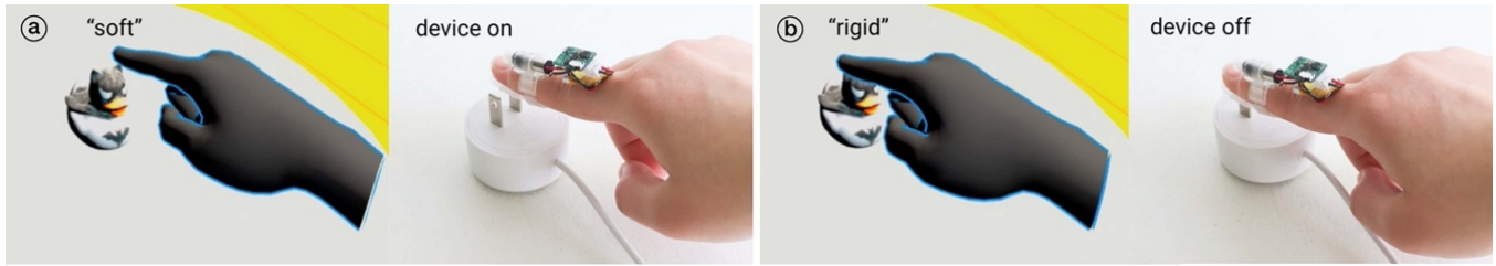
Figure 10: Allowing VR props to switch softness: (a) one ear of the rubber duck feels soft, since our device restricts the fingerpad as the user presses the prop (here, a simple power plug). Conversely, (b) with our device off, the other ear feels hard.
