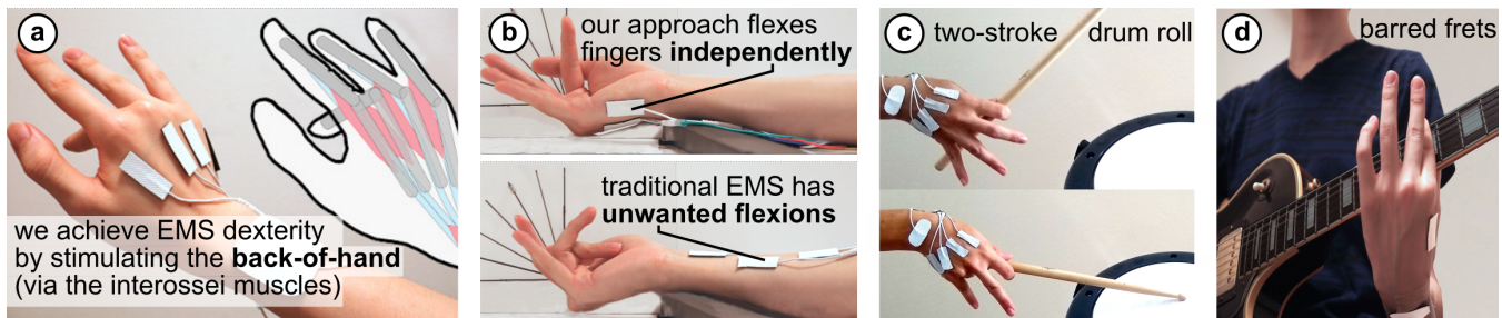
Figure 1: We improved the dexterity of the finger flexion produced by interactive devices based on electrical muscle stimulation (EMS). The key to achieve it is that we discovered a new electrode layout in the back of the hand . Instead of the existing EMS electrode placement, which flexes the fingers via the flexor muscles in the forearm, we stimulate the interossei/lumbricals muscles in the palm. Our technique allows EMS to achieve greater dexterity around the metacarpophalangeal joints (MCP), which we demonstrate in a series of applications, such as (c) a two-stroke drum roll or (d) a barred guitar fret. These examples, as with all others in our paper, were previously impossible with existing EMS electrode layouts.
