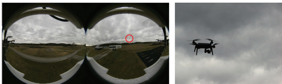
Fig. 14 Example dataset images: synchronous peripheral (left) and central (right) vision images.
