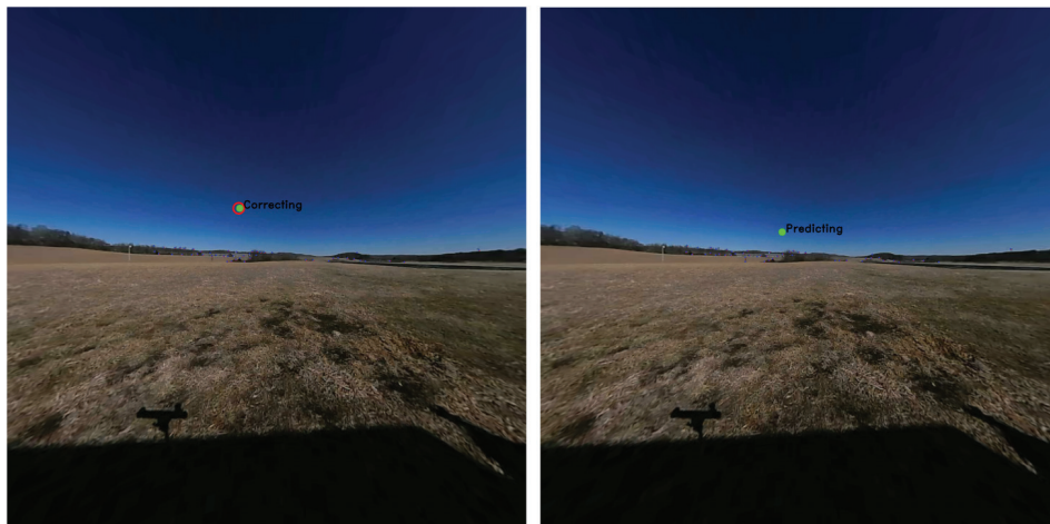
Fig. 7 Two image frames illustrating the results of Kalman-filter-aided optical flow detection.
