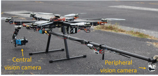
Fig. 2 Peripheral-central vision system setup.
