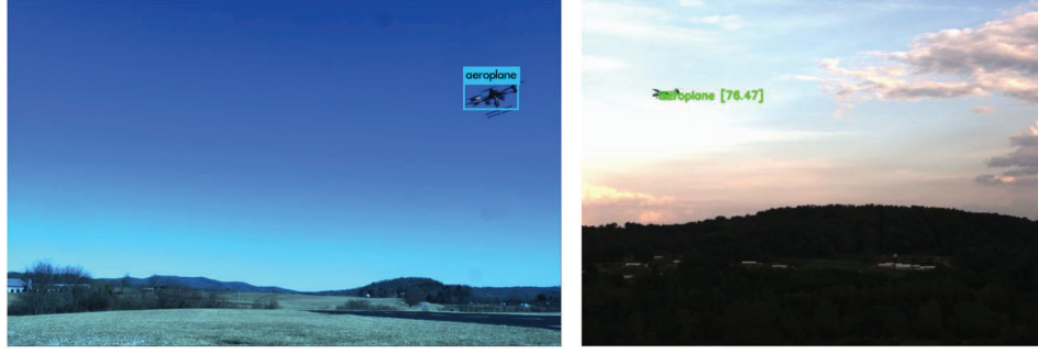
Fig. 9 Example results using COCO-trained YOLOv3.
