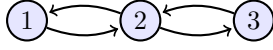
Fig. 1. The figure shows a network where only agent 1 is informative. In Section III, we design an event-triggered algorithm under which all upstream broadcasts along the path 3 \rightarrow 2 \rightarrow 1 stop eventually almost surely.
