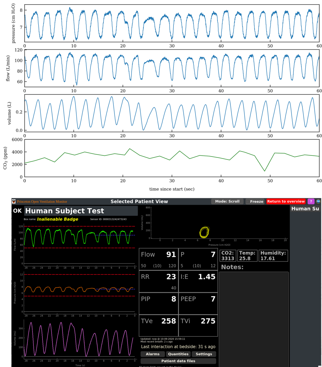
Fig. 10 Respiratory profile of healthy human subject in helmet. Top: Pressure, flow, equivalent tidal volume, and \text{CO}_2 concentration on the expiratory path of a helmet worn by a healthy human subject are shown. Positive flow is defined to be gas leaving the helmet through the expiratory path. Bottom: Derived quantities, including tidal volume, and respiratory rate, are visible on the remote monitoring station (shown here in “drilldown” screen).
