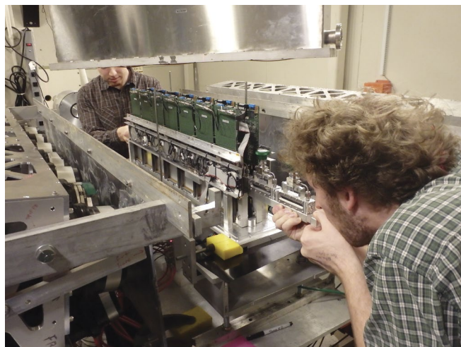
Figure 2. (Left) The target carriage and silicon strip detector arrays used in the kinematically complete measurements of two- and three-body photodisintegration. (Right) Two-dimensional histogram of the energies for the two charged particles detected in coincidence from the photodisintegration of ^3\text{He} in the HIGS experiment, reproduced from Ref. [8]. under the creative common license https://creativecommons.org/licenses/by-nc-nd/4.0/ .
