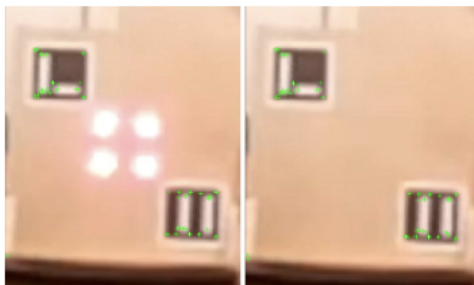
Figure 1. Features extracted using ORB techniques in both LED ON (left image) and LED OFF (right image) states; no key points can be found on LED regions.
