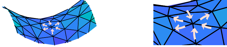
Figure 5: In a piecewise linear approximation of \psi , the saddle points are located at those element vertices \mathbf{v} for which the difference \psi_h(\mathbf{v}) - \psi_h(\mathbf{v}_i) for all its neighboring vertices \mathbf{v}_i changes sign at least four times. The sign of this difference indicates whether the discrete function \psi_h along the element vertices is increasing or decreasing. The point surrounded by the arrows in the figure corresponds to a saddle, as it is a local maximum in one direction and a local minimum in another one. This is reflected by the number of times the arrows change direction.
