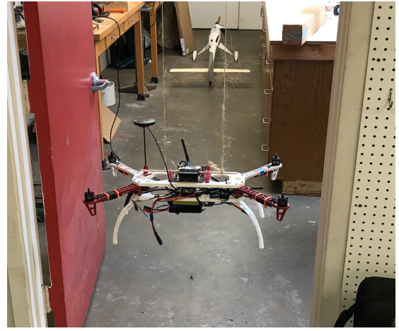
Fig. 6: Measuring the Mass Moment of Inertia of the Asymmetric Quadrotor
