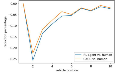
Figure 6. Fuel Consumption of CAV Scenario Compared to HD Scenario.
