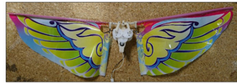
Figure 1. Commercial flapping drone and our modified version with an active pitching mechanism. (a) Commercial flapping wing drone [25]. (b) Modified version of the flapping wing air vehicle with an active mechanism (top view).
