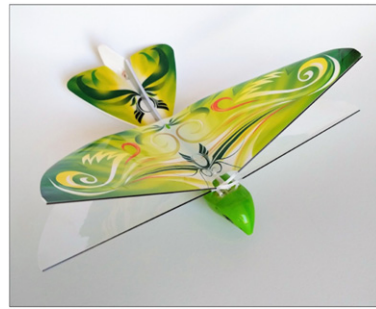
Figure 1. Commercial flapping drone and our modified version with an active pitching mechanism. (a) Commercial flapping wing drone [25]. (b) Modified version of the flapping wing air vehicle with an active mechanism (top view).
