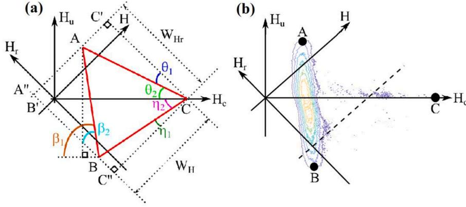
**Fig. 3.** a) Schematic of a FORC diagram showing the points of interest (A, B, and C) in the  $(H_c, H_u)$  plane and correlating the length of lines connecting the  $(H_c, H_u)$  plane onto  $(H_r, H)$  plane. b) Shows the theoretical simulation of a hysteretic system composed of bistable interacting hysterons with a Gaussian distribution of coercivity.
