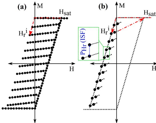
Fig. 2. Schematically compares the required data points for determining the magnetic parameters using (a) the first-order reversal curve (FORC) and (b) the projection method.
