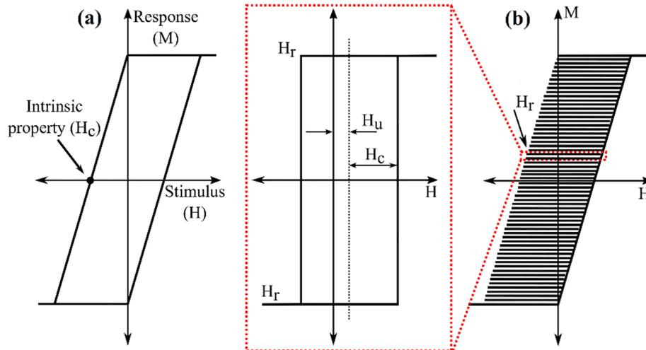
Fig. 1. Schematically illustrating the response/stimulus of hysteretic systems determined using, (a) the hysteresis loop measurement and (b) first-order reversal curve (FORC) measurement. Inset in subfigure (b) shows the response of a hysteron that switches as  $H_r$ , where the  $H_c$  and  $H_u$  are the intrinsic parameter (coercivity) and extrinsic parameter (interaction field), respectively.
