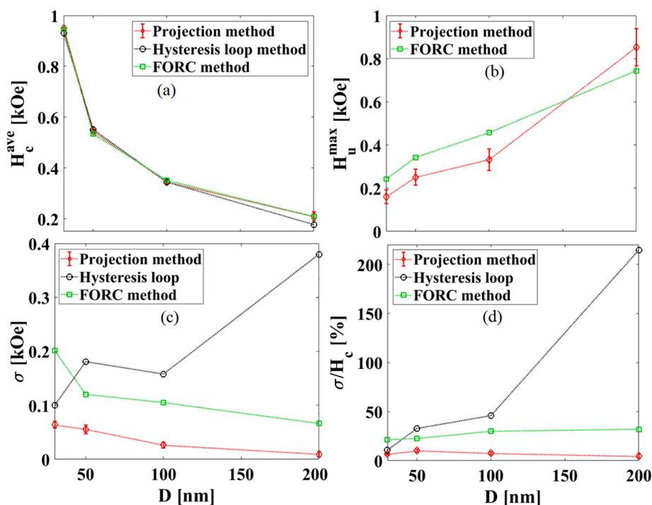
Fig. 4. Comparing the hysteretic parameters for the arrays of MNWs calculated using the hysteresis loop method, FORC method, and the projection method. Aside from subfigure (b), the error bars in other subfigures are in the same size as the symbols.
