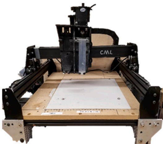
Fig. 1. Syringe 3D printer system used in this study to produce all printed elements.
