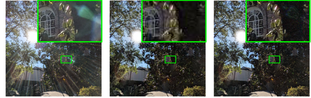
Figure 12. Because lens flares are mostly low-frequency, our algorithm can be trivially extended to high-res inputs. As (a) shows, we downsample (DS) a high-res input (b), predict a flare-free image (c) with our network (CNN), and compute the flare as the difference. This predicted flare is then upsampled (US) and subtracted from the input image to produce a high-res flare-free output (d).
