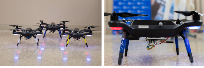
Fig. 9. The photo on the left shows the three 3DR Solo quadcopters used in the indoor and outdoor experiments. The photo on the right shows a close-up view of one quadcopter with its onboard Raspberry Pi 3B+ and custom hardware in the accessory bay.
