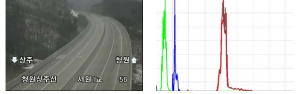
Fig. 2: The histogram plot representing the RGB and gray values of the background image from the road samples.
