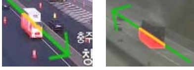
Fig. 1: Sampling road regions from the background image based on the direction of moving vehicles. The red color indicated the sampled road pixels.
