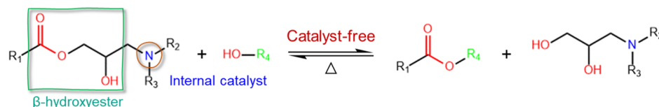
Figure 7. Externally catalyzed transesterification of previous reports and the internal catalysis effect of secondary and tertiary amines of the DCN–PEI network on the transesterification process.
