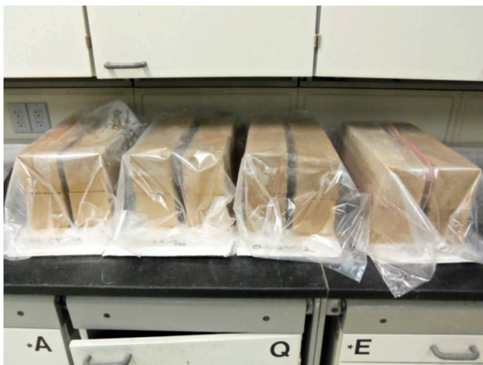
Figure 2. Initial cure of CEBs under plastic sheets.
